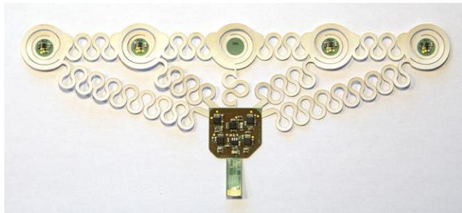
Figure: flexible amplifier circuit for upper arm ECG recording using dry electrodes
